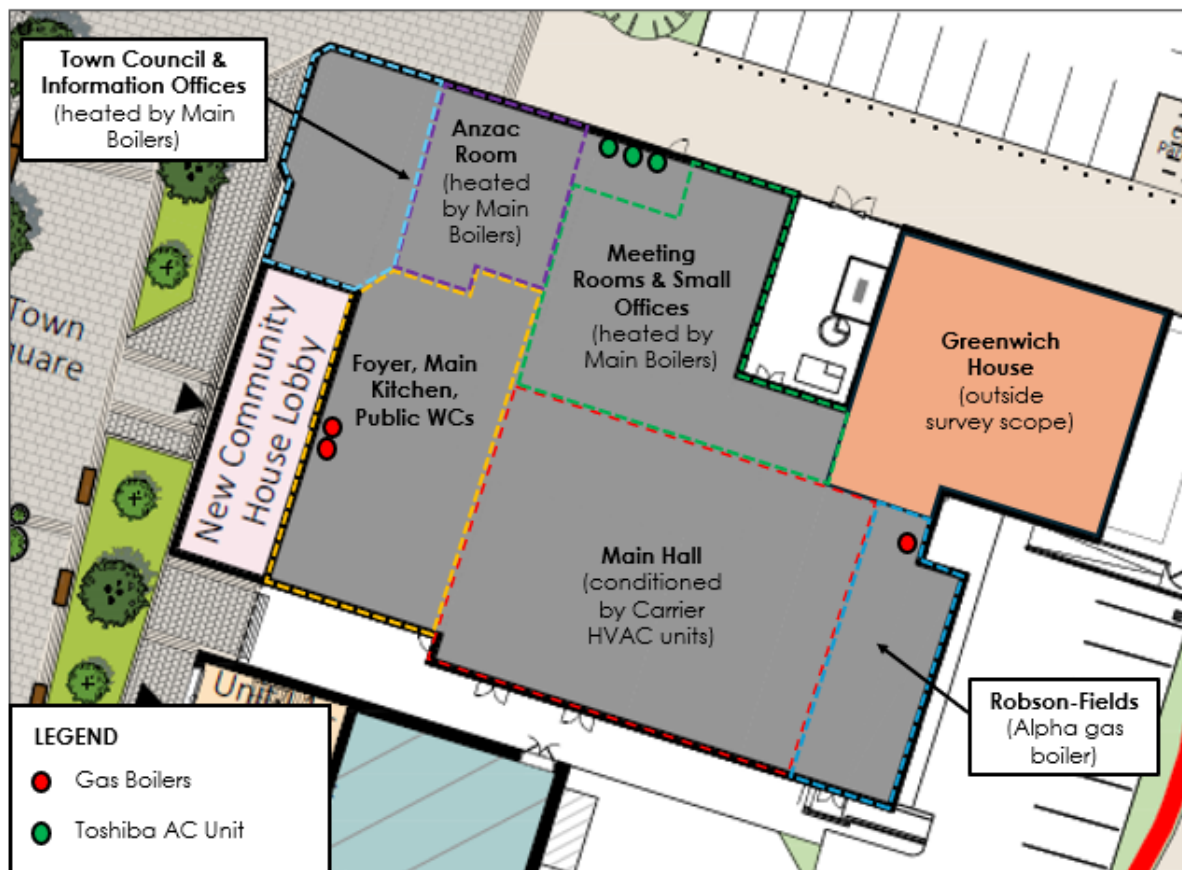
Figure 1 Key areas and heating systems. Adapted from proposed floorplan (Whittam Cox Architects drawing 210211/PL_09)
