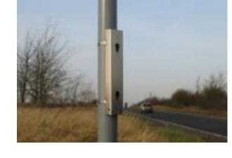
Mount the recorder onto the bracket and secure it with 3 padlocks. 2 padlocks secure the peli-case door, and one secures the peli-case to the pole bracket.
