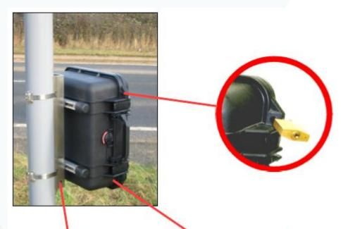
How to fix the radar onto existing street furniture.
