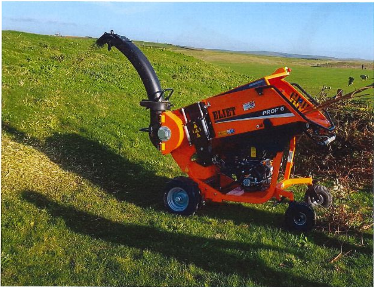
Big hopper opening to fit smaller hedge cuttings
